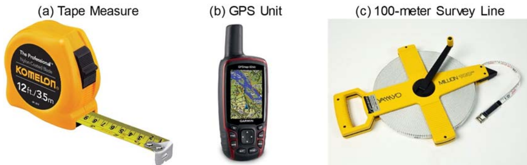
Figure 3: ALT surveys require a measuring tape with a lock (a), a WAAS enabled GPS unit (b), a 100 meter, retractable survey line (c).
