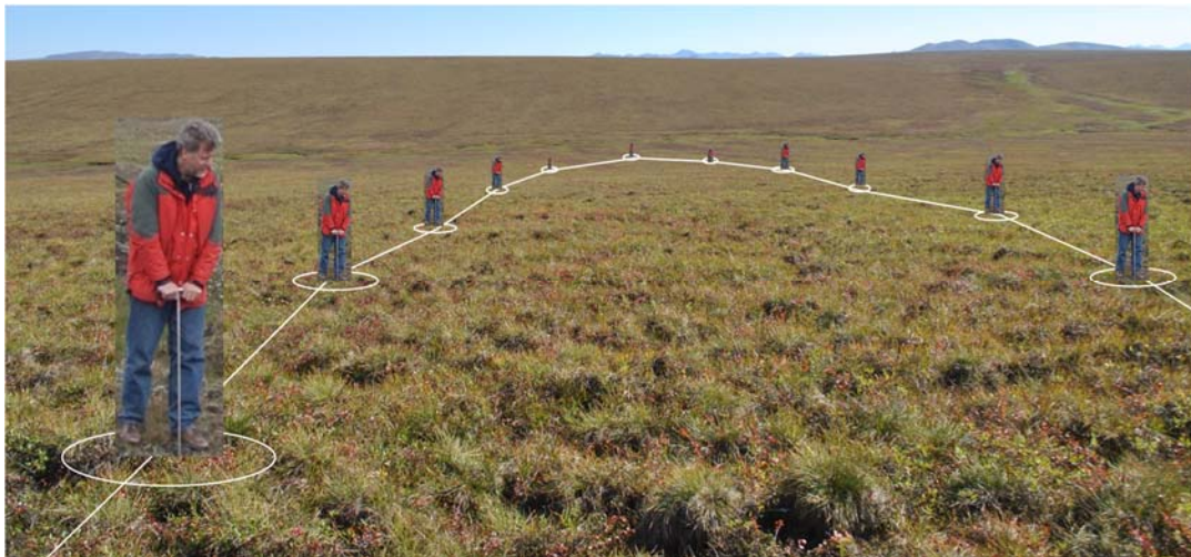
Figure 6: For a Multi-Point Survey, make repeat single point measurements along a path with a spacing of about 10 meters (Toolik Lake, 2015). The path should be a straight line or a loop crossing as many different land units as possible. We do not recommend a grid pattern because it takes so long to set up with minimal benefit for validating radar data. Every point counts. Even a short transect of only 2-3 points can provide valuable validation data.
