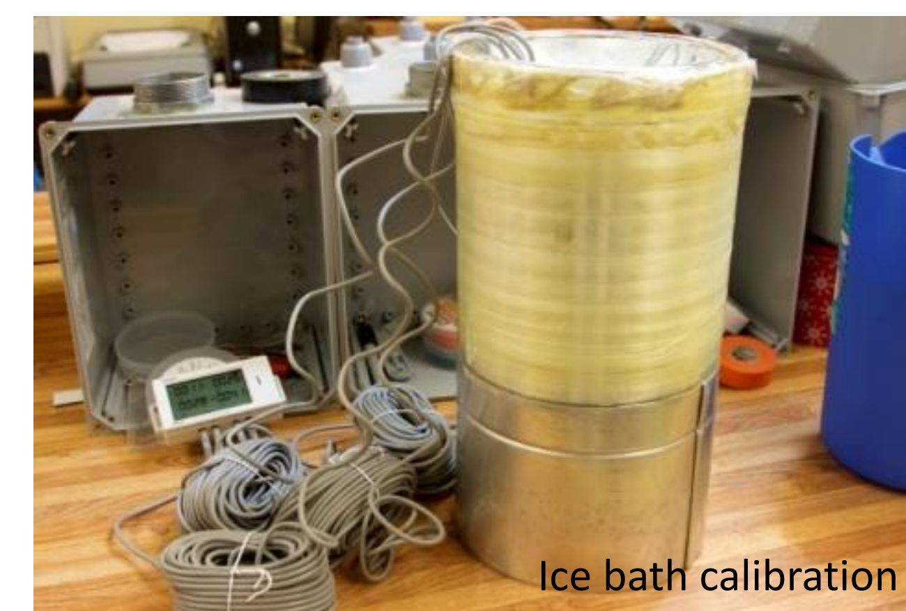
HOBO UX120 4-Channel Analog Data Loggers with two Lithium batteries to support multi-year data collection efforts
