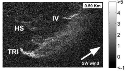
AVIRIS imagery of methane plumes from sub-oceanic seeps off the coast of Santa Barbara CA demonstrate the sensitivity of the instrument to detect methane emissions diffusing through ~10 meters of water
